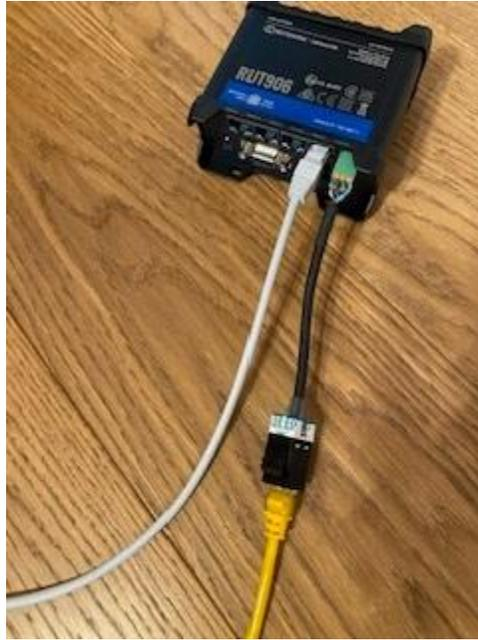
*Photo: Internet cable and modbus cables connected correctly.*
