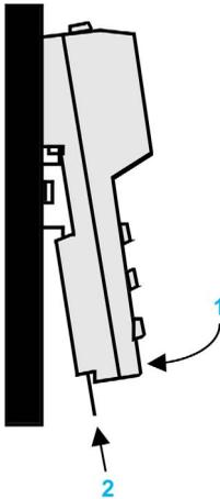
The processor assemblies are mounted on a DIN rail in the same manner as other TSX Momentum assemblies, as follows:
