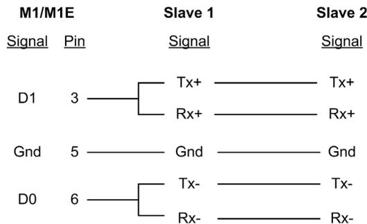
Every other pin on the processor RJ45 serial port connector ([see page 30](#)) is reserved, except for pin number 8, to which a cable shield is connected if you are using shielded wiring.
