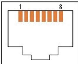
The specified standard—RS232 or RS485—determines the signal assigned to each pin for serial communications:
