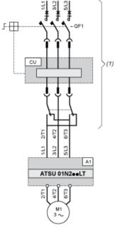
TeSys U with reversing unit Soft start/soft stop unit (1) A1 : QF1 : TeSys U controller-starter TeSys U control unit CU:
