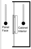
Be sure that heat from surrounding equipment does not cause the panel to exceed its standard operating temperature.
